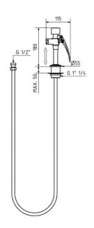
Model: 3120 Bench mounting eyewash with retractable flexible hose.
