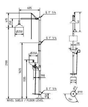
Model: 4250 Floor mounting combination emergency drench shower and eyewash, with additional foot treadle operation.
