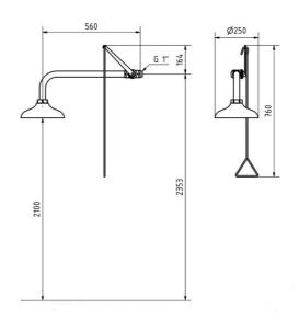
Model: 1110SS Wall mounting emergency drench shower complete with mounting plate.
