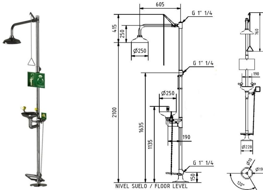
**Model: 4250TI** Floor mounting combination emergency drench shower and eyewash, with additional foot treadle operation. Ideal for germ free, nuclear, medical and food sectors.
