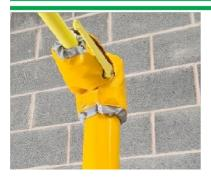
Starting from the top, fit the valve cover #1 onto the shower valve securing with the Velcro flaps & side drawcords. Cover #2 will fit over the Tee section at the top adjacent to cover #1. Ensure the upright foam lagging is inside the drawcords joint before tying securely.
