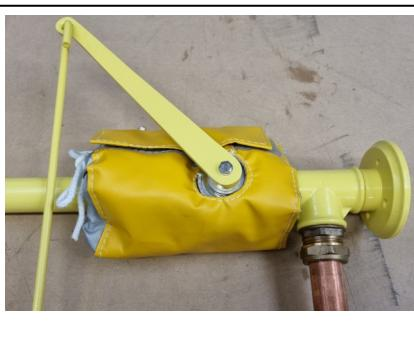
The yellow thermal lagging should be fitted around the valve as shown. Once the lagging has been fitted, secure by pulling the draw strings tightly around the shower outlet pipe. Care should be taken to ensure none of the moving parts are fouled or chaffed by the lagging or the electrical wiring.
